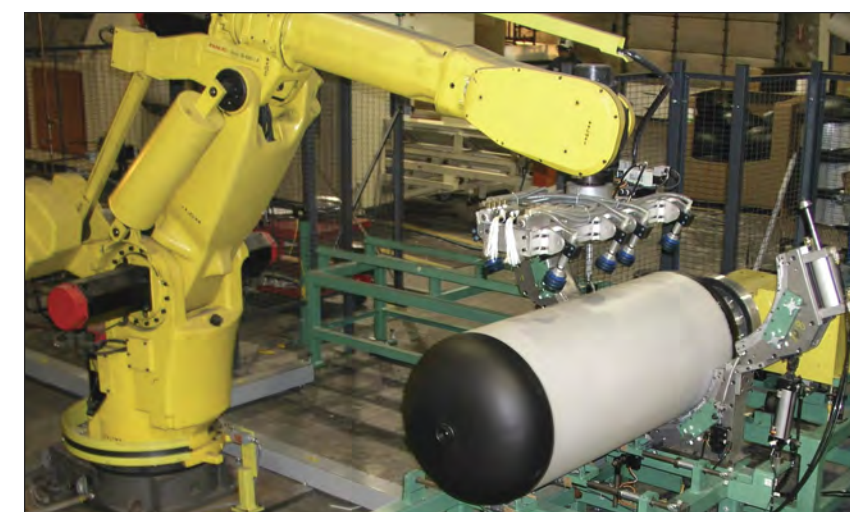
The company's composite tanks are primarily constructed by robot arms. The Flex-Lite tanks are the only composite tanks on the market featuring a double-diaphragm.
