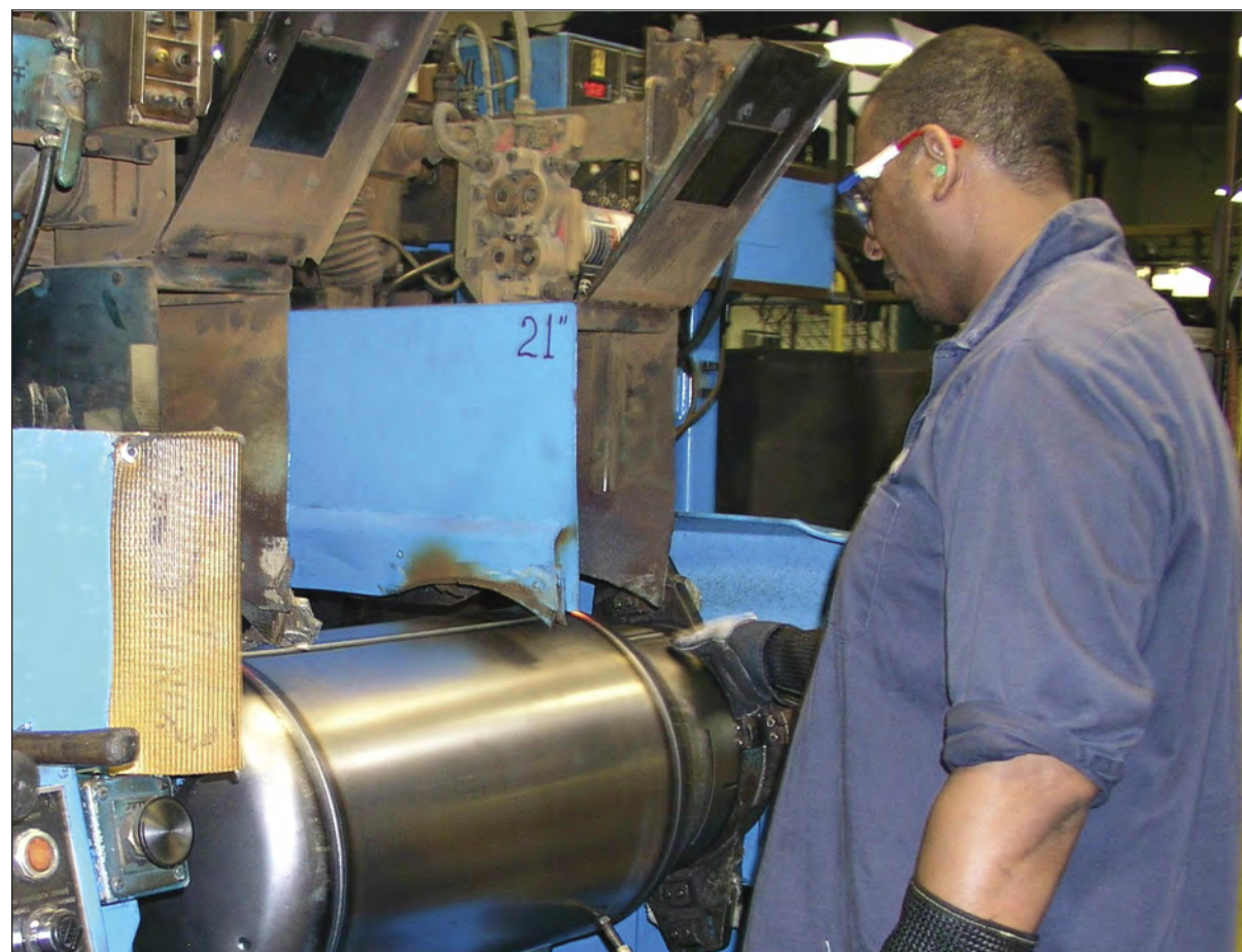
A Flexcon Industries employee welds a steel tank. Each tank is made with a three-piece construction.
