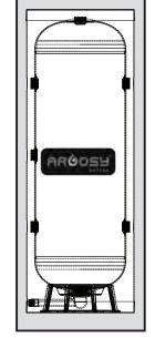
This tank is designed for systems operating up to 180 deg. F at 75 PSI or up to 140 deg. F at 100 PSI. A properly sized pressure relief valve must be installed. This tank must also have a vacuum breaker as any vacuum on the tank will cause it to implode. Failure to install a vacuum breaker will void the warranty.
